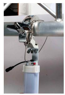
3. Use the large hole on the mounting bracket to affix the LED BP tube to your desired mounting point. Make sure that the mounting hardware (not included) is capable of supporting a minimum point load equal to 10 times the weight of this device. Secure the LED BP tube with safety cable (not included) rated to support at least 12 times the weight of the unit.
