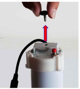
1. Find and remove the thumb screw located on the end of the LED BP tube.
