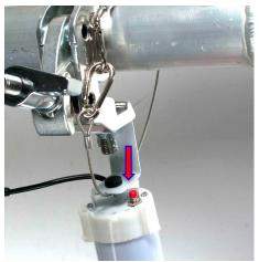
4. **AC POWER OPERATION:** Connect the power supply to the cable lead on the LED BP tube. Plug the power supply into an electrical outlet and press the red button on the end of the LED BP tube to switch the device ON.
